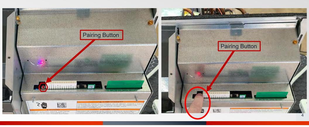
4. Remove the mounting plate of the Amana DS01(x) thermostat. Insert the 2 provided AA batteries. Press and release the white pairing button.
