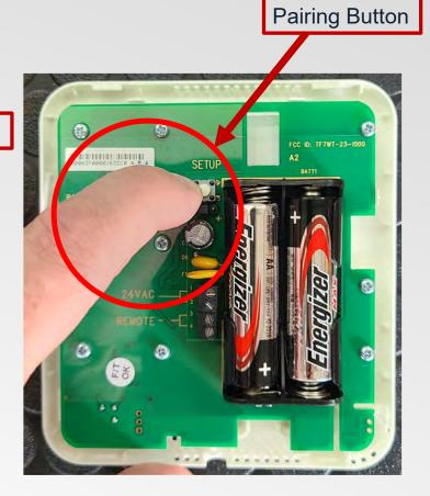
5. The thermostat display will respond with 00 once it pairs to the Amana PTAC unit. Confirm this by pressing the MODE button on the thermostat. The unit will respond to the mode change if paired.
