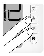
With thermostat powered, press System Mode button until **OFF** is underlined. After OFF mode is confirmed, press and hold BOTH the Up and Down buttons for at least 5 seconds until the screen changes.
