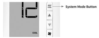
Press System Mode button until desired mode is underlined, after 2 seconds with no button press the underlined system mode is entered.
