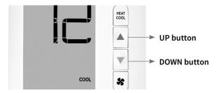
**UP / DOWN** = used for raising or lowering the target set temperature and selecting user options and settings in the display screen.
