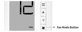
Press Fan Mode button until desired mode is underlined, after 2 seconds with no button press the underlined fan mode is entered.
