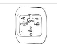
• Feed the wires through the hole in the trim plate and screw the trim plate to the wall
