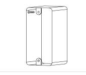
Insert mounting screw into top of junction box until there is approximately 1/8" gap between the screw head and the wall
