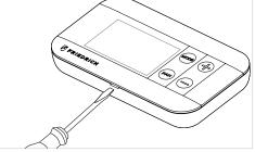
Use a flat head screw driver to separate the front and back housing of the thermostat
