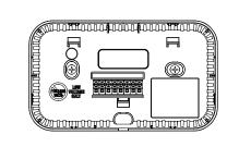
If new mounting holes are needed, mark the placement of the new mounting holes through the thermostat base. Using a 3/16" drill bit, drill the holes you have marked and insert the supplied wall anchors.
