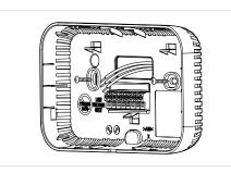
Feed the wires through the hole in the back housing of the thermostat and then screw the back housing to the wall
