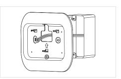
Feed the wires through the hole in the trim plate and hang the trim plate on the top screw
