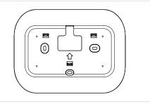
If new mounting holes are needed, mark the placement of the new horizontal mounting holes through the trim plate base. Using a 3/16" drill bit, drill the holes you have marked and insert the supplied wall anchors.
