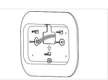
• Feed the wires through the hole in the trim plate and screw the trim plate to the
