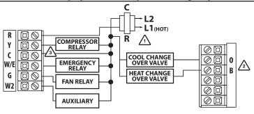
Conventional System 1H/1C, 2H/1C (Heat pump set to "OFF" in tech settings)
