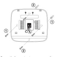
For vertical mount put one screw on the top and one screw on the bottom. For horizontal mount put one screw on the left and one screw on the right.
