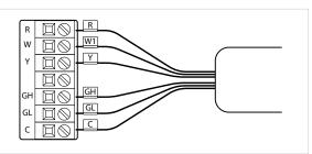
Note 1: If connecting to a Cool only PTAC unit, the W1 and W2 wires will not be used and Installer Settings menu 03 (Available Modes) should be set to "04: Cool Only"
